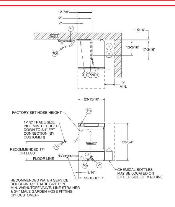
\* THIS SYSTEM REQUIRES THREE POWER WIRES WHICH INCLUDES A CURRENT CARRYING NEUTRAL, AN ADDITIONAL FOURTH WIRE MUST BE PROVIDED FOR MACHINE GROUND.
